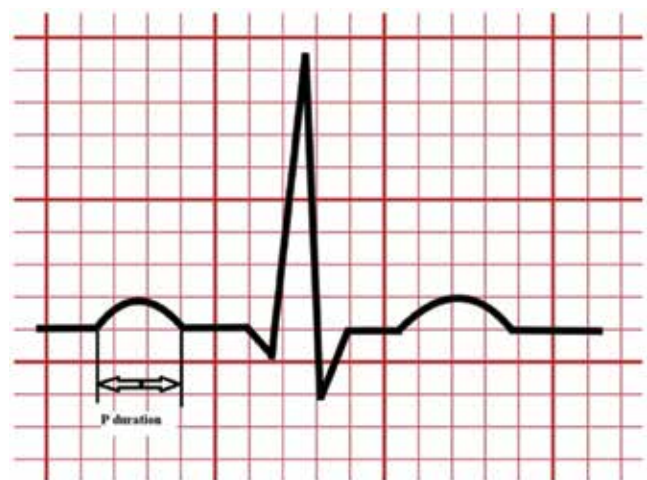
Figure 1. P wave duration measurement
